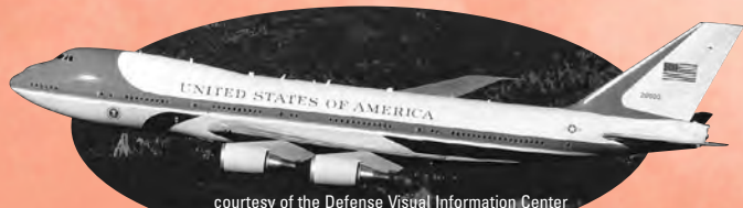
Boeing VC-25A, length: 195 ft., span: 231 ft., speed: 640 m.p.h., range: 7140+ miles
