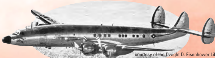
"Columbine III" Lockheed VC-121E, length: 116 ft., span: 123 ft., speed: 330 m.p.h., range: 4000 miles
