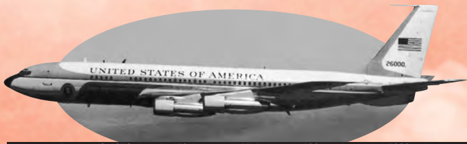
Boeing VC-137C, length: 152 ft., span: 145 ft., speed: 530 m.p.h., range: 5000 miles
