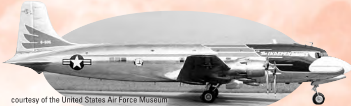
"The Independence" Douglas VC-118, length: 100 ft., span: 117 ft., speed: 360 m.p.h., range: 4400 miles
